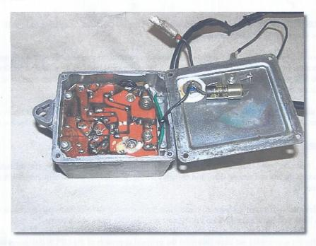
**6)** Depending on the model of the amplifier, the board will have a flat 5 or 6 wire cable attached to it. The 6<sup>th</sup> wire is a Blue/White Tachometer (also known as a Rev-counter) wire and if not present, the Tachometer will be driven off the coil wire. Therefore there is no connection to Pad T on the REOPUS board with 5 wire systems.
